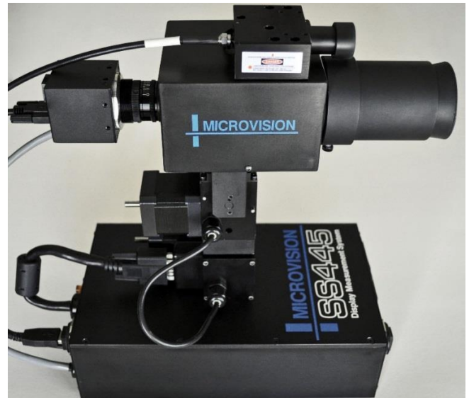
SS445 Shown with CCD Camera and Spectrometer
